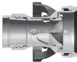
*Coupling halves disconnected*
